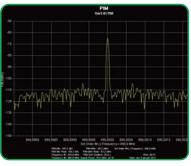
A PIM level of -65.2 dBm has been identified. With a PIM level this high on the Rx channel the receiver will become totally desensitised
