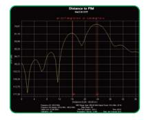
With DTP the PIM source has been identified ~7 m beyond the antenna using markers
